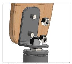
**03** Install each Bracket to Wooden Base as shown in Steps 1 and 2 using supplied Bracket Bolts and Lock Nuts. Note: Maintain tight bolts.
