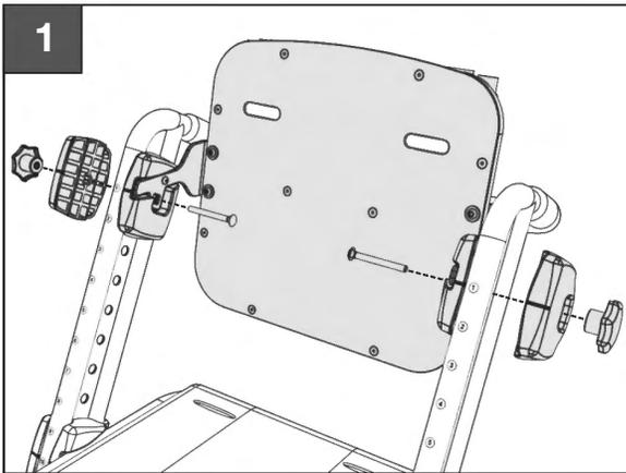
**1.** To adjust the height of the Backrest, begin by unscrewing both Plastic Hand Knobs and remove both Outer Clamps. Then, while supporting the Backrest with one hand, remove each Carriage Bolt from the Inner Clamps. Once both Carriage Bolts are removed, the Backrest will be free to slide along the CatchUp Chair Vertical Frames.
