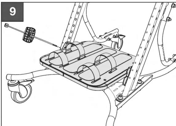
**10.** Next, slide Safety Rod through both Left and Right Vertical Frame holes at Position 20 as shown, ensuring that Safety Rod passes through the Footplate Assembly.
