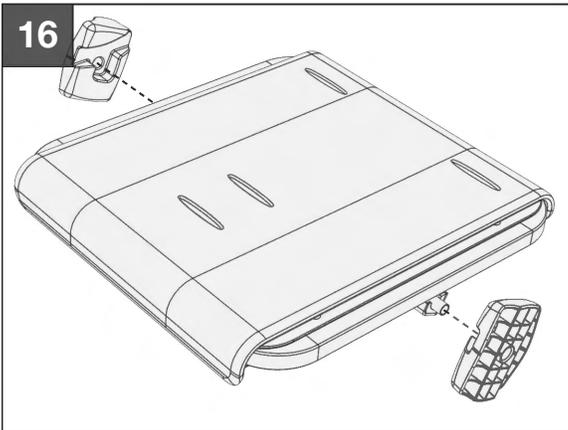
**16.** Mount Inner Clamp Left and Inner Clamp Right to respective sides of the Seatplate as shown here.
