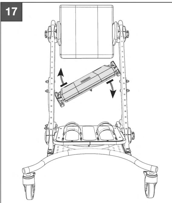
**17.** Insert Seatplate diagonally between Vertical Frames. Then rotate the Seatplate until it is level and both Inner Clamps register between the Vertical Frame Tubes.
