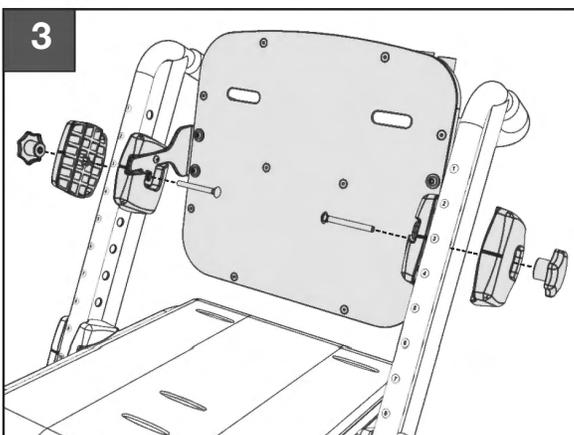
**3.** Re-insert each Carriage Bolt through the two Inner Clamps, then re-attach the two Outer Clamps. Ensure that the Outer Clamps guide-marks are facing forward, then tighten down the two Plastic Hand Knobs.
