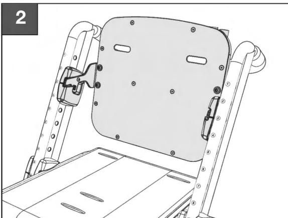
**2.** Reposition the Backrest to the desired height, and be sure that both left and right Inner Clamp guide-marks point to the same Frame Number Position.
