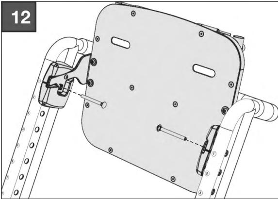
**12.** Position Backrest between the Vertical Frames at Position 1 (top), then insert a Backrest Carriage Bolt through each Backrest Inner Clamp as shown.
