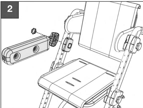
**3.** Tighten down the Plastic Hand Knob to secure the Large Armrest to the CatchUp Chair Frame.
